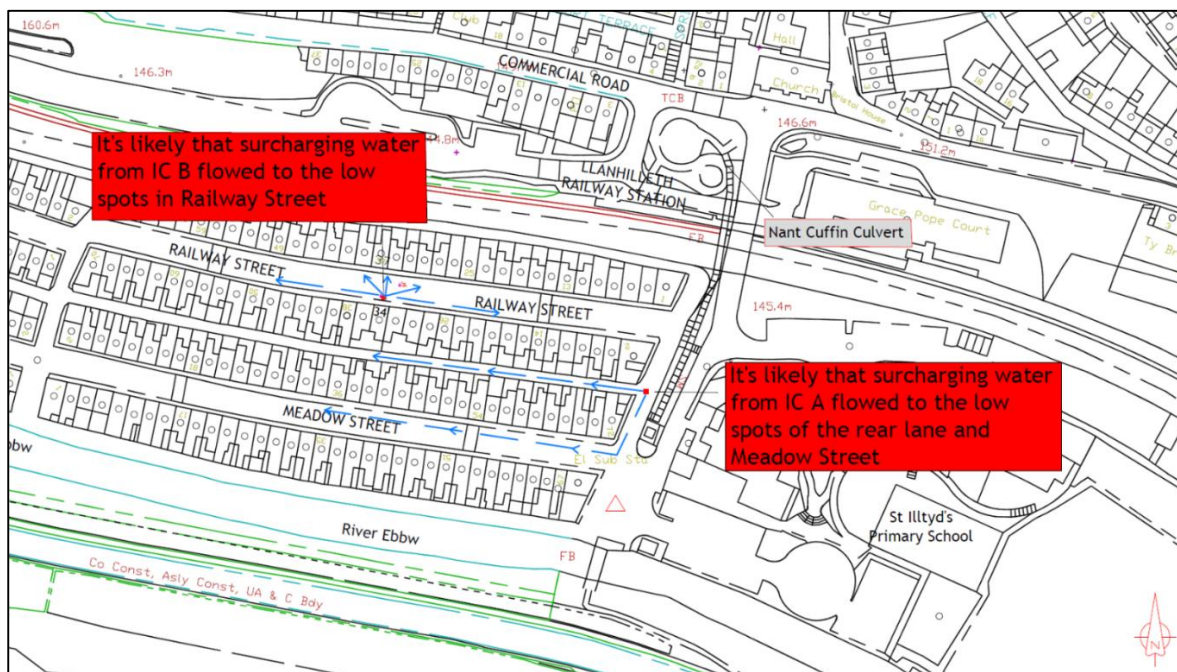
Figure 7 Likely directional flow of surcharging storm water
